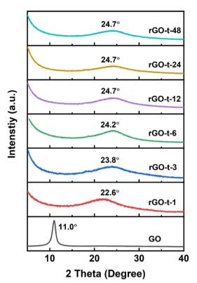
Fig. 4  $\,$  XRD patterns of GO and rGO prepared with various reduction times.
