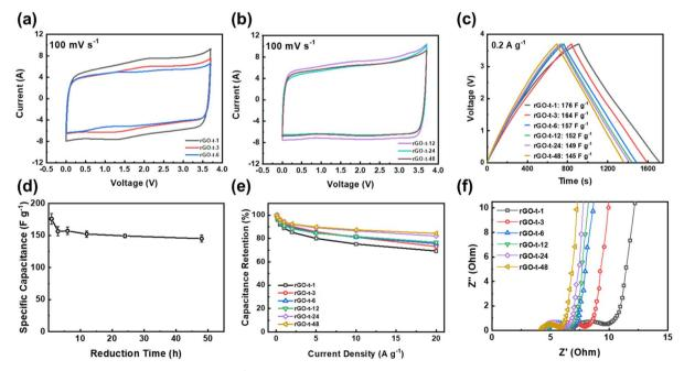
Fig. 8 CV curves at voltage sweep rate of 100 mV s $^{-1}$  of graphene synthesized with reduction time of (a) 1 h, 3 h, and 6 h; (b) 12 h, 24 h, and 48 h; (c) charge–discharge curves, (d) specific capacitance, (e) rate performance, and (f) Nyquist plots of supercapacitors with rGOs synthesized with different reduction times.
