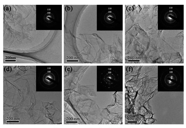
Fig. 1 Low magnification TEM images of rGO with reduction time of (a) 1 h; (b) 3 h; (c) 6 h; (d) 12 h; (e) 24 h; (f) 48 h. Insets are the corresponding selected-area electron diffraction (SAED) patterns. Diffraction rings in the SAED patterns indicate the Bragg reflections corresponding to the (100) and (110) planes of graphene.
