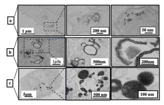
Fig. 12 2D TEM slice images at various magnifications of A431 cells incubated for one day with Fe<sub>3</sub>O<sub>4</sub> nanocrystals coated with dopamine (a), self-assembled in colloidosomes (b) and self-assembled in supraballs (c) ([Fe] = 28  $\mu$ g L<sup>-1</sup>). Source: A. Nicolas-Boluda et al., <sup>57</sup> John Wiley & Sons. Inc.
