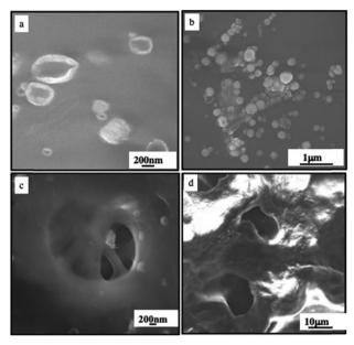
Fig. 16 SEM image of the fresh sheep tendon incubated with colloidosomes (a) and (c) and supraballs (b) and (d) before (a) and (b) and after (c) and (d) irradiated with a NIR laser (10 min at 2 W cm<sup>-2</sup>). Source: A. Nicolas-Boluda et al., 58 John Wiley & Sons. Inc.
