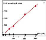
Fig. 3 (a) Extinction spectra of Au "cluster" structures characterized an average size of 198 nm  $\pm$  84 nm recorded experimentally (red curve) and the simulated spectrum (black curve). (b) Variation of the peak wavelength as a function of the assembly size: The black curve illustrates the absorption peak of dispersed Au nanocrystals used as building blocks. The scattering peak represented in the red curve red shifts as the assembly size increases. Source: N. Yang et al., 34 ACS.
