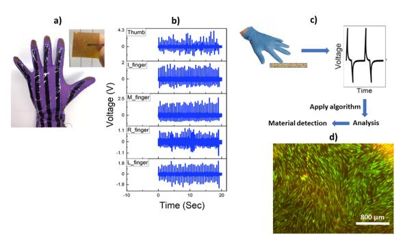
Fig. 7 (a) Image of the TENG sensorized surgical glove with flexible interconnects, (b)  $V_{oc}$  obtained from tapping with the glove on skin, (c) material identification with the TENG mounted glove and (d) fluorescence microscopic image of live human dermal fibroblasts (HDFs) after treatment with the TENG for 48 h, showing excellent biocompatibility.
