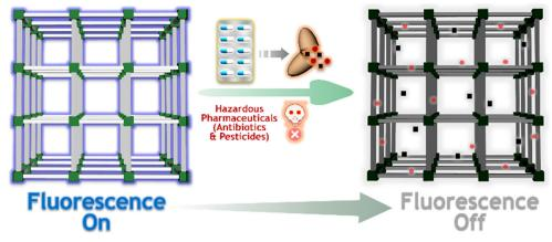
Scheme 1 The schematic representation of the turn-off fluorescence response of iMOF-14C towards hazardous antibiotics and pesticides.
