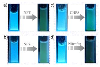
Fig. 2 Photographs of the emission intensity changes of iMOF-14C in water under UV-vis light ( $\lambda$  = 350 nm) upon the addition of an (a) aqueous solution of NFT, (b) aqueous solution of NFZ, (c) aqueous solution of CHPS and (d) aqueous solution of nitrofen, each showing rapid quenching of PL emission intensity.
