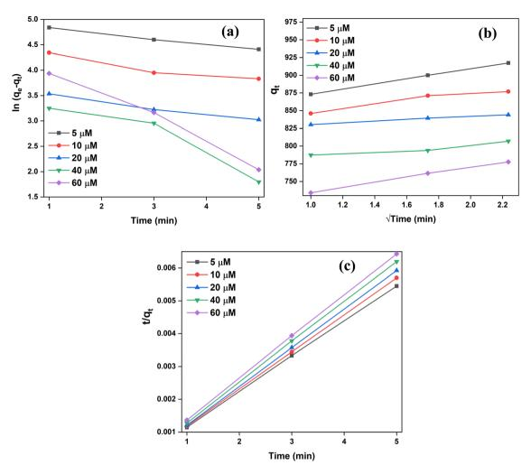
Fig. 8 Adsorption kinetic models studied for varying dye concentrations (5-60 μM) and a constant adsorbent dose (0.1 g/100 mL): (a) pseudo-firstorder, (b) intra-particle diffusion and (c) pseudo-second-order.
