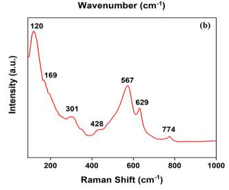
Fig. 2 (a) FTIR spectra and (b) Raman spectra of SnO<sub>2</sub> NPs.
