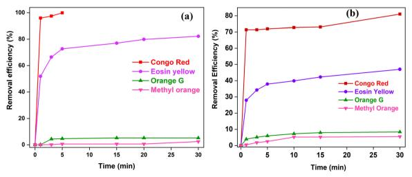
Fig. 5 Adsorption of four anionic dyes at a concentration of 5  $\mu$ M using (a) 0.1 g/100 mL of SnO<sub>2</sub> NPs and (b) 0.3 g SnO<sub>2</sub>@SA beads.
