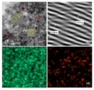
Fig. 4 (a) Enlarged view of TEM images of SnO<sub>2</sub> NPs showing various lattice fringes marked in a red circle; (b) magnified view of red circle 1 from image (a); and panels (c) and (d) show the elemental mapping of SnO<sub>2</sub> NPs with Sn and O in green and red colors, respectively.
