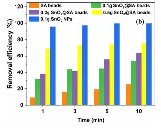
Fig. 10 (a) Various compositions of SnO<sub>2</sub>@SA beads for CR dye adsorption, and (b) their comparative analysis through a bar diagram.
