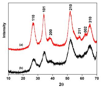
Fig. 1  $\,$  XRD spectra of (a)  $\rm SnO_2$  NPs in a powder form and (b)  $\rm SnO_2$  NPs encapsulated within SA beads.
