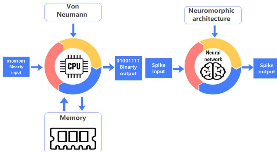
Fig. 2 Von Neumann architecture vs. neuromorphic architecture.
