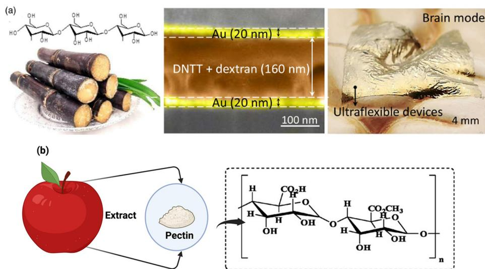
Fig. 4 Biomaterial-based artificial synaptic devices with ultraflexibility: (a) ultraflexible organic synaptic transistors based on dextran,<sup>48–50</sup> (b) organic synaptic transistors based on pectin from apples.
