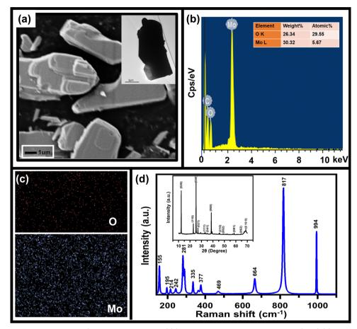
Fig. 1 Characterization of as-synthesized  $MoO_3$  powder as seen using (a) SEM micrograph along with TEM image (inset), (b) EDX spectrum for elemental confirmation (inset: elemental composition table), (c) elemental composition, and (d) Raman spectrum and XRD pattern (inset).
