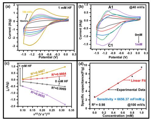
Fig. 2 CV graph of  $MoO_3$  at GCE with (a) 1 mM HF, (b) 0 mM, 0.2 mM, 0.5 mM, 0.8 mM, and 1.0 mM HF in 0.5 M LiClO<sub>4</sub> in PC, (c) variation of current density ( $j_p$ ) vs.  $v^{1/2}$  graph with and without HF, and (d) variation of specific capacitance with concentration of HF including raw data and linear fit.
