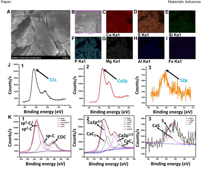
Fig. 1 (A) SEM image of CaC<sub>2</sub> at 10 μm. (B)-(I) Distribution of all elements and their core-level studies based on SEM mapping. (J1-3) XPS data. (K1-3) Fitted XPS data for carbon, calcium, and sulfur distribution.
