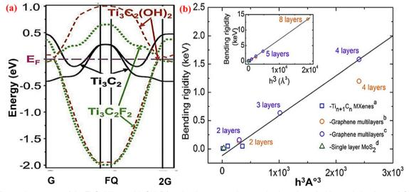
Fig. 5 (a) Electronic structure of the Ti<sub>3</sub>C<sub>2</sub> MXene with OH, F functional groups, and no termination adopted with permission from ref. 96. Copyright 2011 John Wiley and Sons. (b) The bending rigidity of the  $Ti_{n+1}C_n$  MXene,  $MoS_2$ , and graphene multilayer in relation to their thickness. Reprinted with permission from ref. 83. Copyright 2018 Elsevier.
