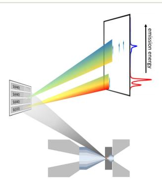
Fig. 1 Representation of the scattering geometry for a two-color experiment using one Si(333) and three Si(440) reflections measuring the Fe K $\alpha$  (red) and K $\beta$  emission (blue), respectively.
