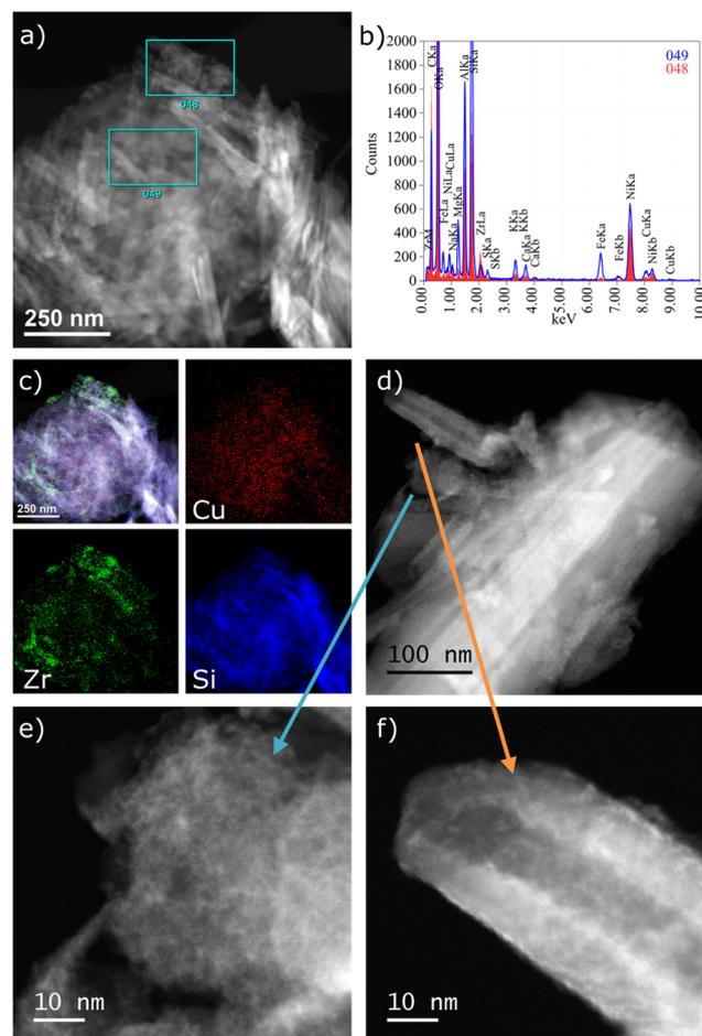
**Fig. 2** (a) Overview HAADF-STEM image, (b) EDX spectra from regions marked in (a), (c) EDX elemental maps of CuZr/5A, (d) more detailed HAADF-STEM image with Zr containing regions highlighted in (e), showing a rather large amorphous particle, and (f), showing bright smaller clusters adhering to the support surface.
