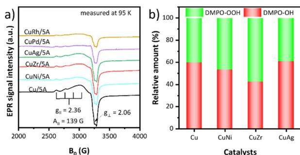
Fig. 3 (a) EPR spectra of the prepared catalysts recorded at 95 K. (b) H<sub>2</sub>O<sub>2</sub> activation abilities of catalysts.
