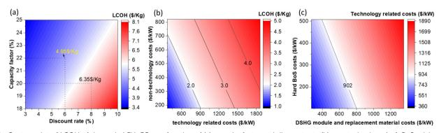
Fig. 5 Contour plot of LCOH of decoupled PV-EC as a function of (a) capacity factor and discount rate (b) non-technology (soft BoS + labour) and technology (hard BoS + DSHG module + replacement materials) related costs. (c) Contour plot of technology related costs as a function of Hard BoS and DSHG module + replacement materials cost.
