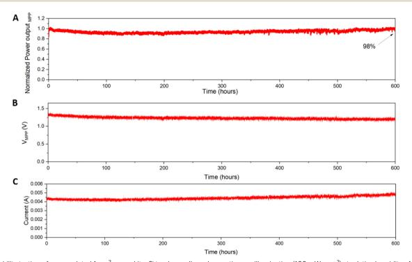
Fig. 5 Stability testing of encapsulated 1 cm<sup>2</sup> perovskite-Si tandem cells under continuous illumination (100 mW cm<sup>-2</sup>) at relative humidity of  $60 \pm 20\%$ at room temperature. Maximum power point tracking of (A) power output, (B) voltage ( $V_{MPP}$ ) at the maximum power point and (C) current to the starting value at the maximum power.
