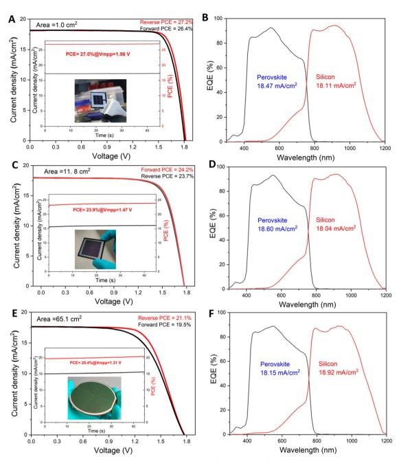
Fig. 4 Performance of champion tandem devices of different sizes. (A, C and E) light J-V and (B, D and F) external quantum efficiency (EQE) of the perovskite-Si tandem devices of (A and B) 1 cm<sup>2</sup>, (C and D) 11.8 cm<sup>2</sup>, and (E and F) 65.1 cm<sup>2</sup>. Insets show the photographs of the fabricated tandem devices and their steady-state current densities and steady-state PCEs at fixed voltages near their maximum power points.
