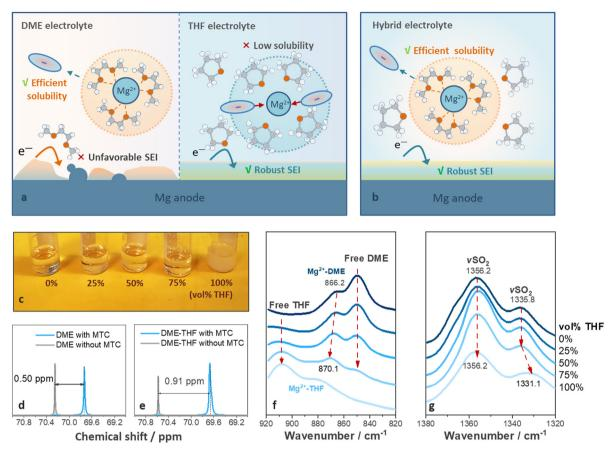
Fig. 1 Schematic illustration of structure of (a) single-solvent and (b) hybrid electrolytes. (c) Digital photographs of DME, DME-THF (25–75 vol% THF), and THF electrolytes. <sup>13</sup>C NMR spectra of methylene carbons in DME (d) without and (e) with THF (75 vol% THF). (f) and (q) Ex situ FT-IR spectra of DME, DME-THF (25-75 vol% THF), and THF electrolytes.
