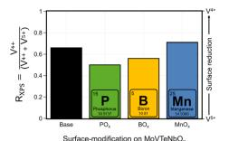
Fig. 5 Effect of surface deposition of BO<sub>x</sub>, PO<sub>x</sub>, MnO<sub>x</sub> on the oxidation state of V in the near-surface region of MoVTeNbOx after catalysis (spent); the ratio  $R_{XPS}$  between reduced  $V^{4+}$  species and the sum of  $V^{4+}$  and  $V^{5+}$  calculated from the XPS spectra in the of  $V_{2p_{3/2}}$ region (see Fig. SI16 and SI17† for more details) is shown.
