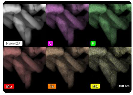
Fig. 3 STEM-HAADF images of PO<sub>x</sub> surface-modified MoVTeNbO<sub>x</sub> after catalysis (spent sample): EDX-mappings show element dispersion of both bulk elements (Mo, V, Te, Nb) and the additionally deposited phosphorus; the images of the fresh sample are shown in Fig. SI8;† the mappingspectra of both samples are attached in Fig. SI9 and SI10.†
