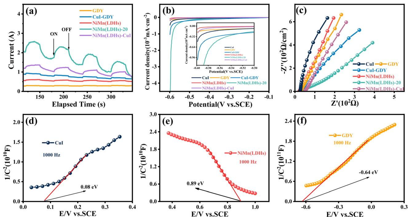
Fig. 10 (a) Transient photocurrent response of GDY, CuI-GDY, NiMn(LDHs), NiMn(LDHs)-CuI, NiMn(LDHs)-20; (b) LSV curves and (c) EIS spectra of CuI, GDY, CuI-GDY, NiMn(LDHs), NiMn(LDHs)-CuI, NiMn(LDHs)-20; (d–f) Mott-Schottky plots of CuI, NiMn(LDHs), and GDY.
