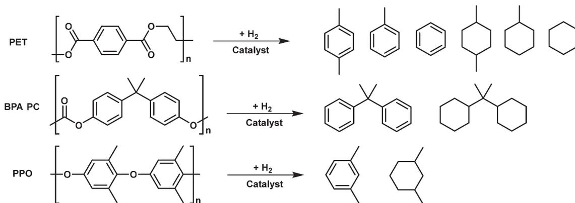
Fig. 12 Hydrodeoxygenation of PET, BAP PC and PPO.
