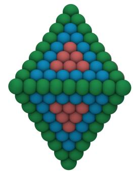
Fig. 9 Interaction heatmap of an oxygen probe atom with a pristine 3 nm octahedral NP. Interaction strengths for the surface atoms are calculated by averaging over interaction points on the SASA nearest to each surface atom. Interaction strength: green > blue > red.
