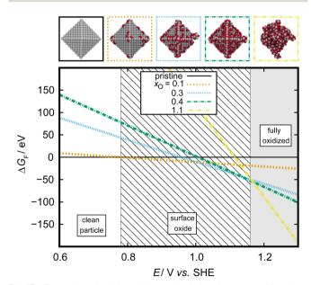
Fig. 13 Electrochemical phase diagram depicting the most stable adsorbate structures on a 3 nm octahedral Pt NP. Adsorbate structures are characterized by their O:Pt ratio,  $x_{O}$ , as outlined in Section 3.1. Adapted from Kirchhoff et al.26
