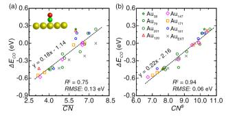
Fig. 2 Comparison of CO adsorption energy trends on Au clusters and extended surface obtained with DFT and a (a)  $\overline{\text{CN}}$ - or (b)  $\text{CN}^{\alpha}$ -based descriptor method. Reprinted with permission from Ma and Xin, Phys. Rev. Lett., 2017, 118, 036101. Copyright 2017 by the American Physical Society.
