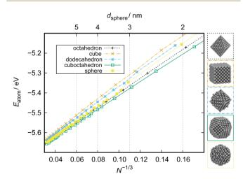
Fig. 10 Stability of cuboctahedral, octahedral, spherical, dodecahedral, and cubic Pt NPs as a function of particle size obtained from ReaxFF calculations. N: number of atoms in a particle. The key diameter of the spherical particle,  $d_{\text{sphere}}$ , is given on top. Bottom: Illustration of NP structures of ca. 3 nm size. Adapted from Kirchhoff et al.<sup>24</sup>
