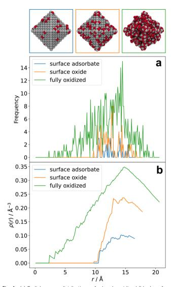
Fig. 4 (a) Radial oxygen distributions of a barely oxidized (blue), surface oxidized (orange), and fully oxidized (green) 3 nm octahedral Pt NPs obtained from ReaxFF GCMC calculations. (b) Integrated, normalized radial oxygen density distributions of the same structures.
