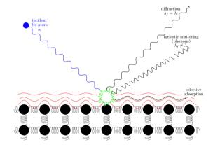
Fig. 10 A helium atom scattering experiment. The helium atom can scatter elastically to give a diffraction pattern, inelastically to provide information about surface dynamics or be adsorbed on the surface
