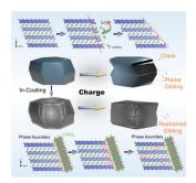
Enhanced mechanical strength of a highly de-lithiated single-crystal Ni-rich cathode to suppress irreversible planar gliding
