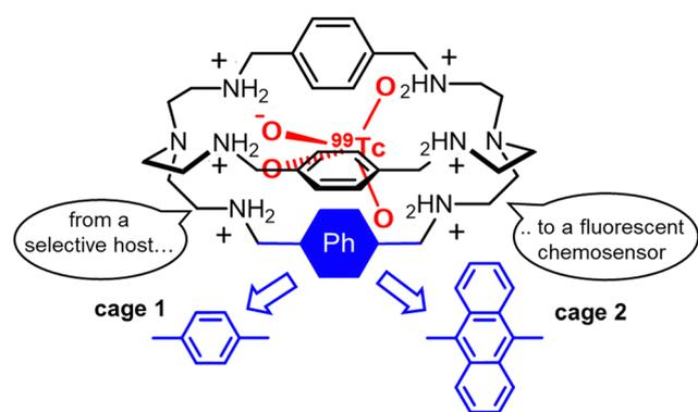
Fig. 1 Schematized structures of the hexaprotonated bistren cages **1** and **2**, employed in the capture and sensing of the pertechnetate anion in aqueous solution.
