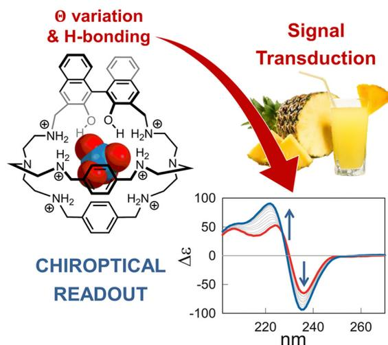
Fig. 2 Schematized structure of the inclusion complex formed by the hexaprotonated cage **3** and perrhenate in aqueous solution. The cage was applied in the chiroptical sensing of this target anion (as surrogate for pertechnetate) in complex aqueous media, such as fruit juice and the artificial urine medium. Reproduced from *Chem. Commun.*, 2022, **58**, 3897.<sup>53</sup>
