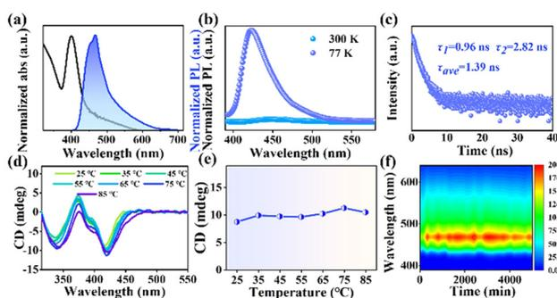
Fig. 2 (a) UV absorption and PL emission spectra of  $(R\text{-MPEA})_4\text{AgBiBr}_8$  NBs, (b) Temperature-dependent PL spectra, (c) time-resolved PL decays spectra, (d) temperature-dependent CD spectra, (e) corresponding CD intensity at CD peaks of 420 nm and (f) PL intensity of  $(R\text{-MPEA})_4\text{AgBiBr}_8$  NBs under ambient conditions with the relative humidity of  $\text{RH} = 65 \pm 5\%$ .
