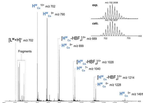
Fig. 2 ESI-MS spectrum of 10  $\mu\text{M}$   $\text{H}^{\text{W}}_{\text{Co}}$  in  $\text{H}_2\text{O}$ , the 10+ to 5+ cage charge states are marked. Fragmentation products and cage species resulting from the loss of  $\text{HBF}_4$  are also observed. The experimental vs. calculated  $m/z$  values for  $\text{H}^{\text{W}}_{\text{Co}}^{10+}$  are shown in the inset.
