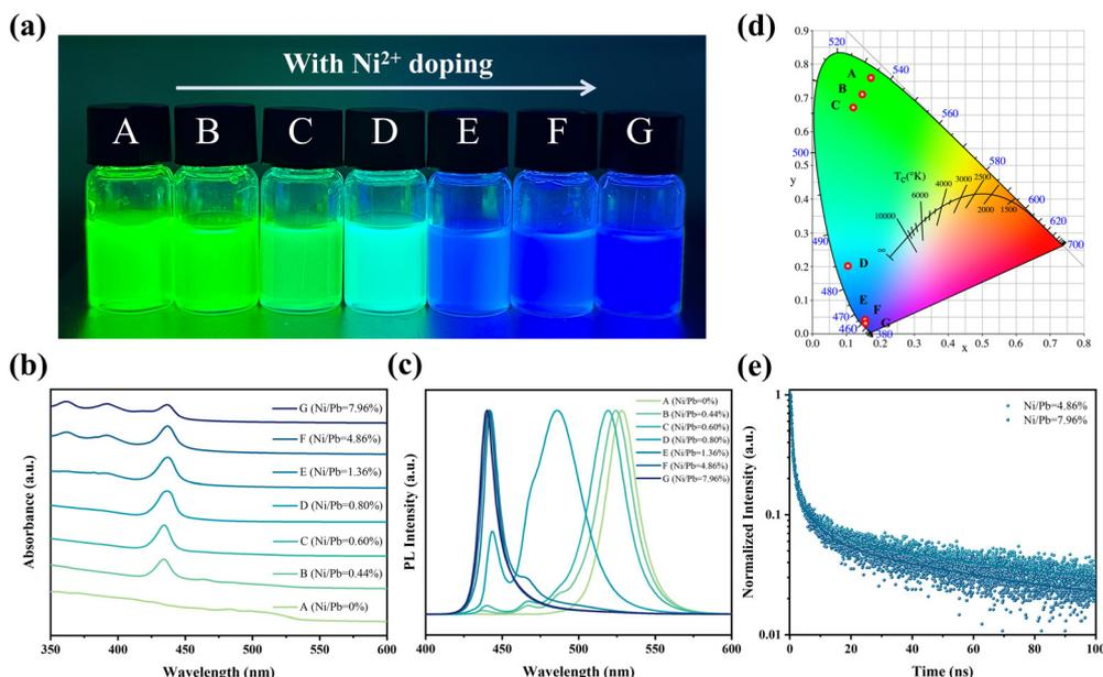
Fig. 1 (a) Images under UV-light (365 nm), (b) UV-vis absorption spectra, (c) PL spectra, and (d) CIE coordinates for  $\text{Ni}^{2+}$  doped  $\text{FAPbBr}_3$  QDs. (e) PL decay curves of deep blue QD solutions with Ni/Pb ratios of 4.86% and 7.96% (measured emission wavelength: 442 nm).
