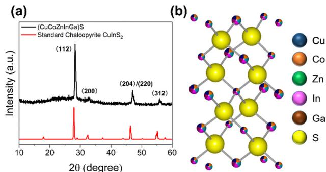
**Fig. 1** Figure of (a) powder X-ray diffraction pattern of thin film (CoCuZn-Ga)S with reference to standard chalcopyrite (CuInS<sub>2</sub>, ICSD: 66865). (b) The crystal structure of HE chalcopyrite ( $a = b = 5.52$ ,  $c = 11.13$ ,  $\alpha = \beta = \gamma = 90^\circ$ ).
