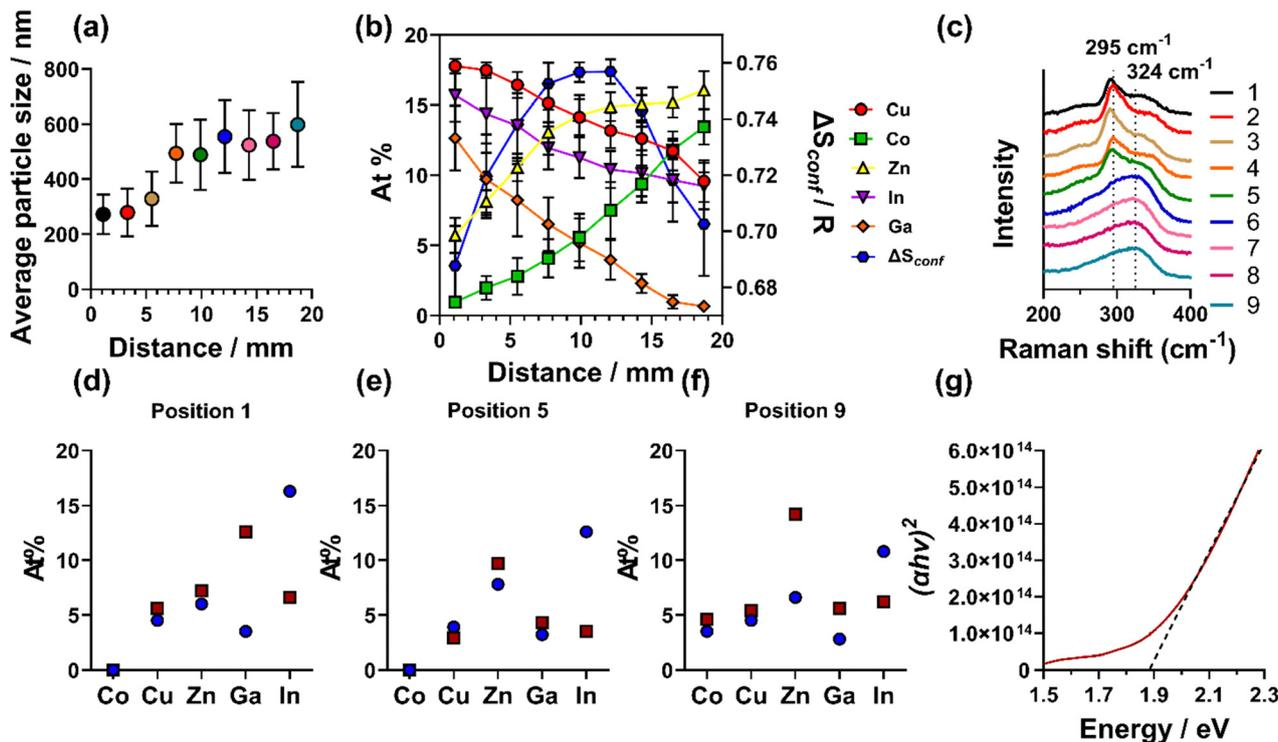
Fig. 3 (a) Particle size distribution analysis across the film of the SEM images (Fig. S8, ESI<sup>†</sup>). (b) SEM-EDX elemental analysis across the film. (c) Raman spectra obtained across the film (d)–(f) XPS (blue circles) vs. HAXPES (red squares) atomic abundance determined from (d) the initial 1–3 mm, (e) 9–11 mm and (f) 17–20 mm of the film. (g) Tauc plot of the UV-Vis spectra shown in Fig. S23 (ESI<sup>†</sup>).
