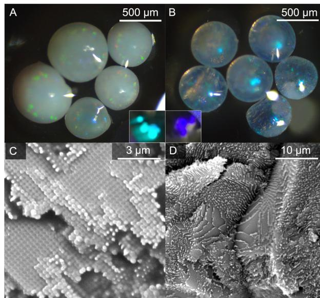
Fig. 2 Optical micrographs of (A) 370PC  $C_{s}PbBr_{3}$  and (B) 190PC  $C_{s}PbCl_{1.5}Br_{1.5}$  microbead hybrids exposed to light from above in silicone oil with insets of hybrids illuminated with  $\lambda_{ex} = 365$  nm. SEM of (C) 370PC  $C_{s}PbBr_{3}$  and (D) 190PC  $C_{s}PbCl_{1.5}Br_{1.5}$ .
