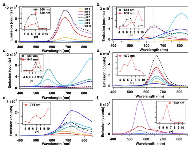
**Fig. 2** Changes in emission intensities of (a) DNA-1, (b) DNA-2, (c) DNA-3, (d) DNA-4, (e) DNA-5, and (f) DNA-6 when prepared at pH 4 (yellow), 5 (red), 6 (purple), 7 (dashed black), 8 (teal), 9 (light blue), and 10 (dark blue). Insets show change in emission intensity at a specific wavelength (indicated by dashed vertical grey line in the main graph) as a function of pH. Emission spectra recorded two days after  $\text{NaBH}_4$  reduction.
