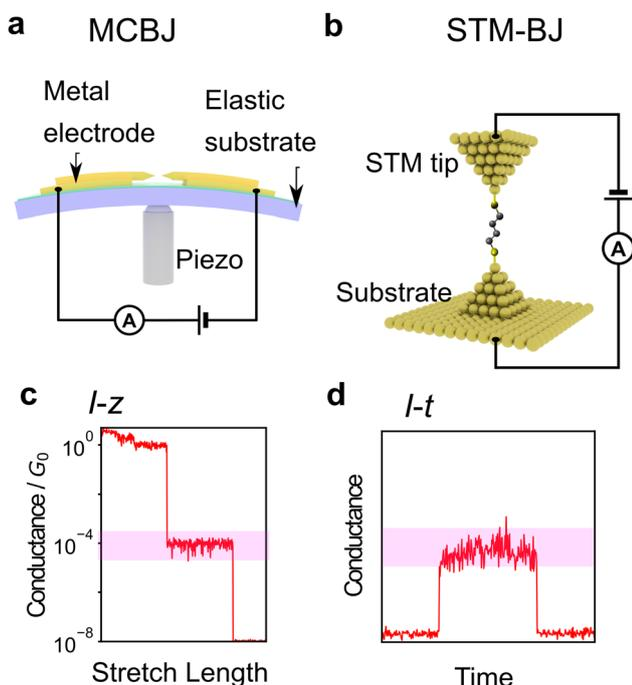
Fig. 2 (a and b) Schematic illustration of setup of single-molecule measurement. (a) MCBJ, (b) STM-BJ (c and d) typical conductance profile image of single-molecule measurement using (c)  $I$ - $z$  method and (d)  $I$ - $t$  method. Red highlights represent single-molecule conductance.
