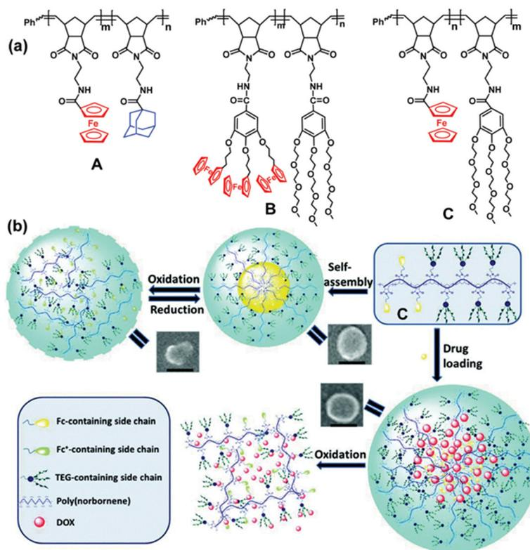
Fig. 22 (a) ROMP-synthesized metallopolymers A, B and C containing ferrocenes. A forms an amphiphile upon  $\beta$ -cyclodextrin addition, and B and C are amphiphiles that self-assembles in redox-responsive micelle (b) Redox-controlled micelles of C for the encapsulation/release of drugs upon redox switch of the ferrocene units; SEM images are shown (scale bar: 100 nm). Reproduced with permission from ref. 163. Copyright 2019 Royal Society of Chemistry.
