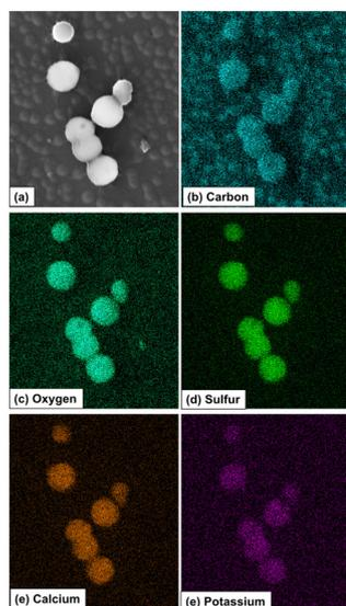
**Fig. 21** SEM/EDS elemental mapping profiles of the vesosomes resulting from self-assembling triazolylferrocenyl dendrimers in water. Reproduced from ref. 151. Copyright 2021 American Chemical Society.
