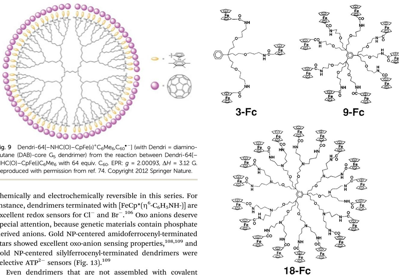
Fig. 9 Dendri-64[–NHC(O)–CpFe(II) $^+$ C<sub>6</sub>Me<sub>6</sub>,C<sub>60</sub> $^{* -}$ ] (with Dendri = diamino-butane (DAB)-core  $G_5$  dendrimer) from the reaction between Dendri-64[–NHC(O)–CpFe(I)C<sub>6</sub>Me<sub>6</sub> with 64 equiv. C<sub>60</sub>. EPR:  $g = 2.00093$ ,  $\Delta H = 3.12$  G. Reproduced with permission from ref. 74. Copyright 2012 Springer Nature.
