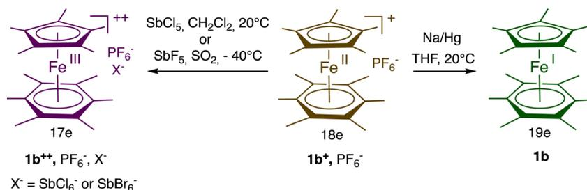
Scheme 3 Synthesis of the stable, fully methylated mixed sandwich Fe complexes with 17 and 19 valence electrons [ $d^5$ , Fe(III) resp.  $d^7$ , Fe(I)] that are both redox catalysts and electrocatalysts.
