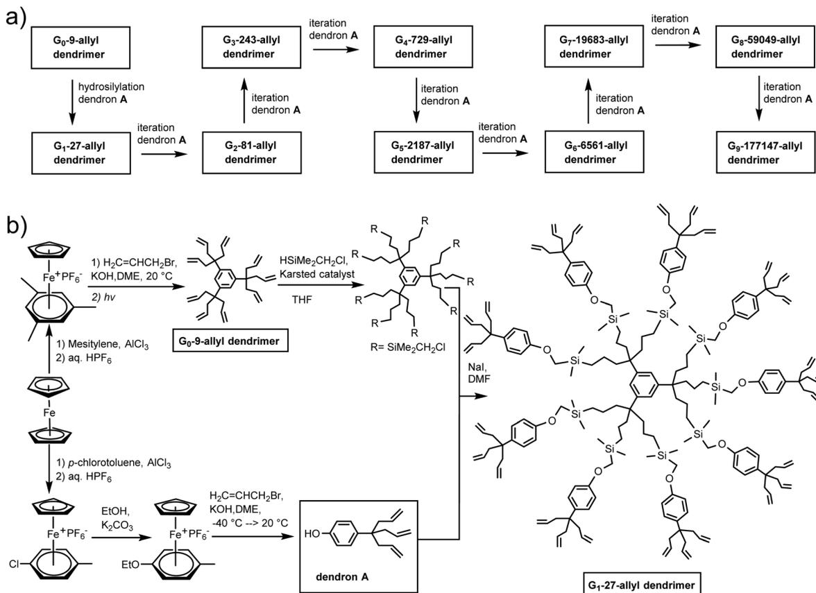
Scheme 6 CpFe<sup>+</sup>-induced arene activation for the synthesis of the G<sub>0</sub>-9-allyl dendritic core and dendron A towards the multiple-generation divergent construction of large poly-allyl-terminated dendrimers following 1 → 3 branching until the 9th generation.
