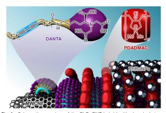
Schematic overview of the RhRuCNT hybrid with chemical structures of DANTA and PDADMAC
