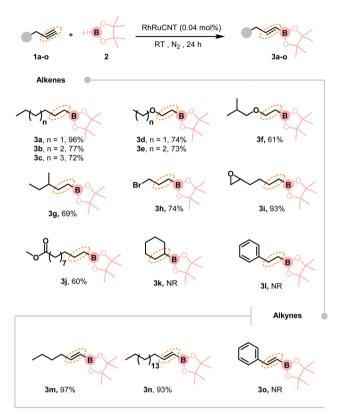
Scheme 2 Substrate scope for the hydroboration. Reaction conditions: Substrate (1.0 mmol), 2 (1.1 mmol), RhRuCNT (0.04 mol%), room temperature (RT), inert atmosphere (N2), neat, 24 h. Isolated yields are shown. NR: no reaction
