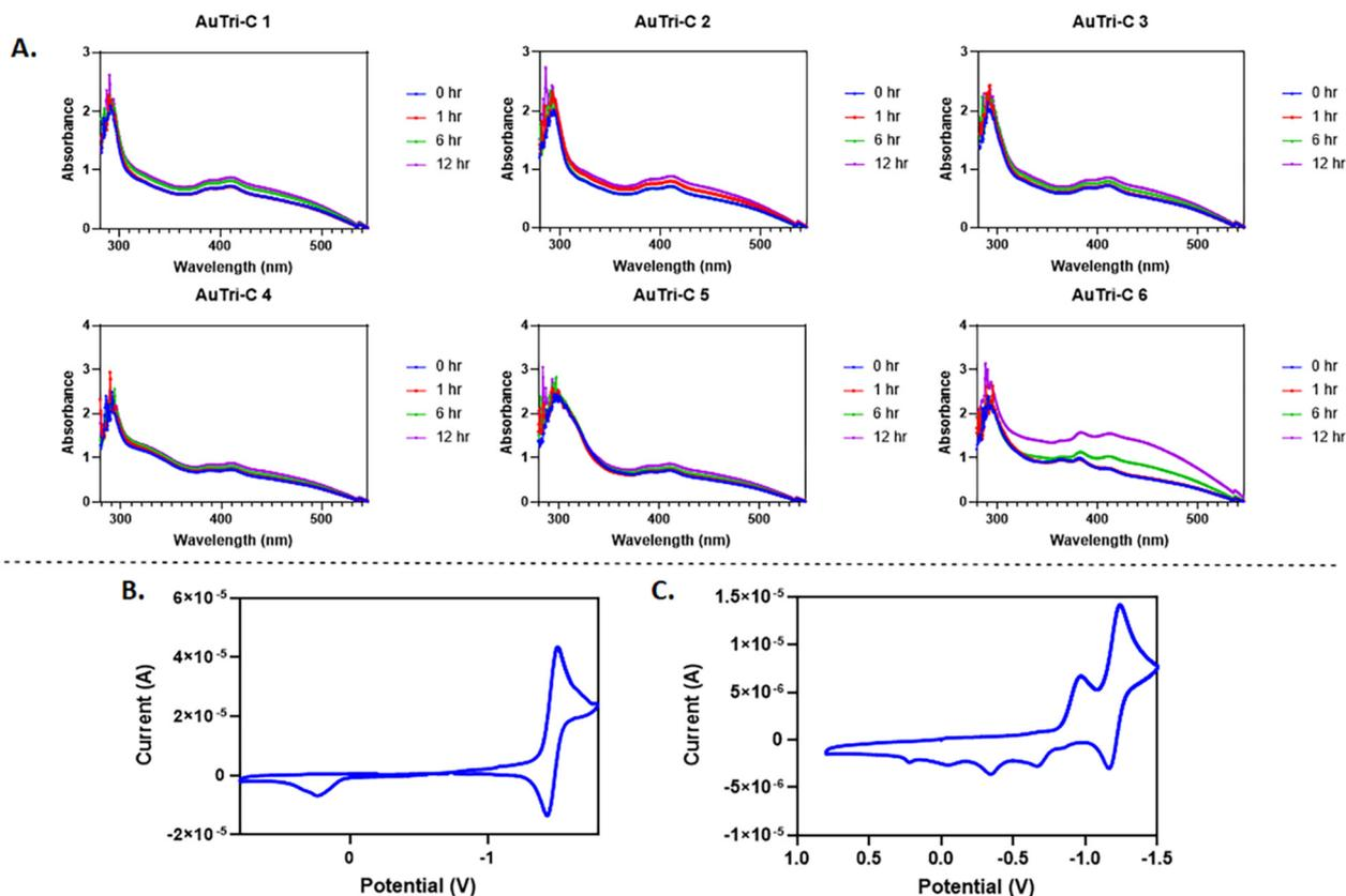
Fig. 2 (A) UV-vis absorption spectra of AuTri-C complexes in biologically relevant media, DMEM at 37 °C, final concentration of the complexes 50  $\mu$ M. (B and C) Cyclic voltammogram recorded at a platinum electrode in DMSO solution of 5 mM AuTri-C-5 or AuTri-C-6 with 0.10 M  $N(\text{Bu})_4\text{PF}_6$  supporting electrolyte at a scan rate of 0.1 V  $\text{s}^{-1}$  using Ag/AgCl reference electrode at RT.
