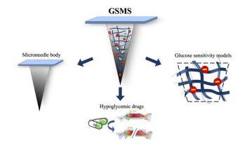
Fig. 1 Composition of glucose-sensitive microneedle system (GSMS).
