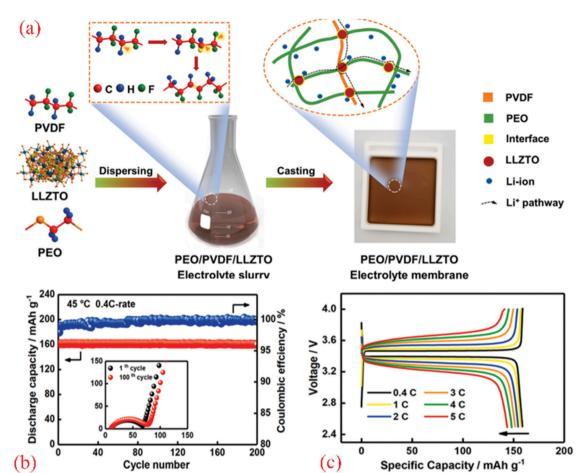
Fig. 21 (a) Fabrication process of the PLFF (PEO/PVDF/LLZTO/LiTFSI) solid composite electrolyte. (b) Cycling performances at 0.4C and 45 °C and the impedance of LiFePO<sub>4</sub>/Li cell cycling with PLFY. (c) Different rates of galvanostatic charge-discharge profiles of LiFePO<sub>4</sub>/PLFY/Li cells under 45 °C. 358 Reproduced with permission from Elsevier. 358
