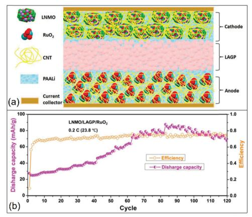
Fig. 19 (a) Schematic illustration of the full lithium-ion solid-state battery using LNMO/CNT/PAALi as the cathode, LAGP as the solid electrolyte, and RuO<sub>2</sub>/CNT/PAALi as the anode, where both sides were sputtered with gold as current collectors. (b) Discharge capacity and efficiency of LNMO/LAGP/  $RuO_2$  at room temperature at 0.2C using PAALi as a binder. <sup>408</sup> Reproduced with permission from The Royal Society of Chemistry, UK. <sup>408</sup>
