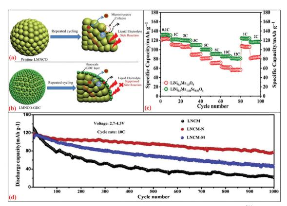
Fig. 8 Schematic illustrations of (a) pristine LMNCO interfacial side reactions with liquid electrolyte after repeated cycling<sup>244</sup> and (b) GDC coating layer acts as a protection layer to suppress the unwanted interfacial side reactions after repeated cycling. 245 (c) Rate capability for LNMO and LNMSO cathode for 0.1–12C. (d) Cycling performances for LNCM, LNCM-N, LNCM-M at C-rate of 10C. 246 Reproduced with permissions from Elsevier. 244–246
