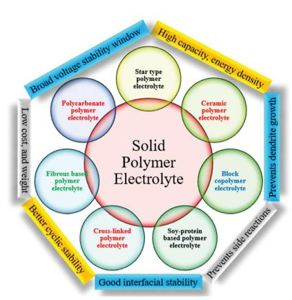
Different types of solid polymer-based electrolytes and their corresponding performances.
