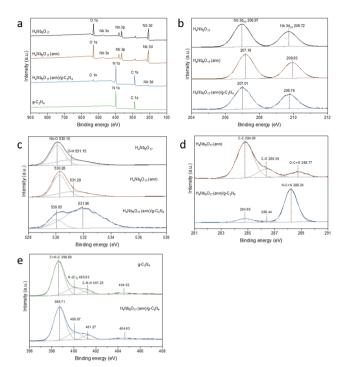
Fig. 7 XPS survey spectrum (a), Nb 3d (b), 1s (c), C 1s (d) and N 1s (e) spectra of H<sub>4</sub>Nb<sub>6</sub>O<sub>17</sub> before and after annealing and H<sub>4</sub>Nb<sub>6</sub>O<sub>17</sub> (ann)/g-C<sub>3</sub>N<sub>4</sub> composite samples
