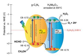
Fig. 10 Schematic illustration of the band levels and charge transfer pathways in the H<sub>4</sub>Nb<sub>6</sub>O<sub>17</sub> (ann)/g-C<sub>3</sub>N<sub>4</sub> composite.
