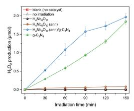
Fig. 8 Time-dependent photocatalytic H<sub>2</sub>O<sub>2</sub> production of the samples under visible light irradiation
