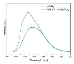
PL spectra of g-C<sub>3</sub>N<sub>4</sub> and the H<sub>4</sub>Nb<sub>6</sub>O<sub>17</sub> (ann)/g-C<sub>3</sub>N<sub>4</sub> composite.
