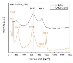
Raman spectra of H<sub>4</sub>Nb<sub>6</sub>O<sub>17</sub> before and after annealing
