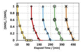
Fig. 4 Recyclability experiments of MIL88-A in the UVA/MIL88-A/PS/ SMX system. Experimental conditions:  $[SMX]_0 = 5 \text{ mg L}^{-1}$ ;  $[PS]_0 = 2$ mM; [MIL88-A] = 125 mg L<sup>-1</sup>; error bars are calculated as  $ts/\sqrt{n}$ , where absent bars fall within the symbols.
