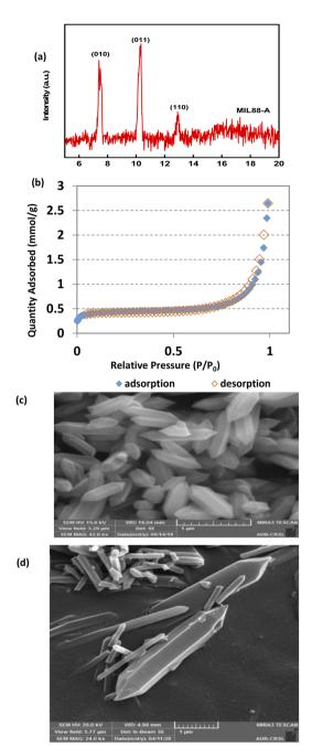
Fig. 1 SEQ Fig. \\* ARABIC Characterization of synthesized MIL88-A: (a) XRD diffraction pattern, (b) BET adsorption/desorption isotherms 71, and (c and d) SEM of crystals at different magnifications.71
