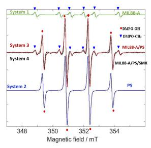
Fig. 11 EPR spectra. Green – simulated EPR spectrum for trapped methyl radicals. aN =1.58 mT and aH =2.28 mT. Blue – simulated EPR spectrum for trapped hydroxyl radicals. aN = 1.49 mT and aH = 1.49 mT. Red – the sum of the above two simulated trapped radical spectra. Black – experimental EPR spectrum under the following experimental conditions: [PS] = 2.5 mM, [MIL88-A] = 12.5 mg L $^{-1}$ , and [DMPO] = 100 mM.
