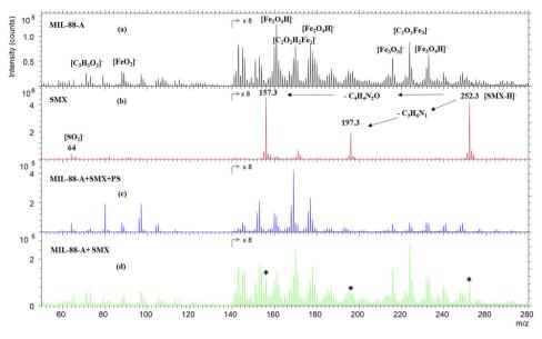
Fig. 2 TOF-SIMS negative spectra of (a) MIL88-A as prepared, (b) SMX powder, (c) MIL88-A after use in the presence of SMX and PS, and (d) MIL88-A+ 5% SMX powder. The areas of the spectra are multiplied by 8 for visual purposes. \* The characteristic peaks of the SMX molecule.
