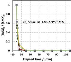
Fig. 7 Effect of [NaCl] =  $200-20000 \text{ mg L}^{-1}$  on the degradation of SMX as a function of time (min): (a) in the UVA/MIL88-A/PS/SMX system and (b) in the solar/MIL88-A/PS/SMX system. Experimental conditions:  $[SMX]_0 = 5 \text{ mg L}^{-1}$ ,  $[PS]_0 = 2 \text{ mM}$ , and  $[MIL88-A]_0 = 125 \text{ mg}$  $L^{-1}$ . Error bars are calculated as  $ts/\sqrt{n}$ , where absent bars fall within the symbols
