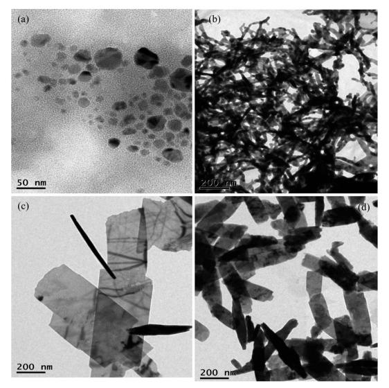
TEM image of Cu nanosheets synthesized at (a) 0.5 M (b) 1 M (c) 2 M and (d) 3 M NaOH concentrations
