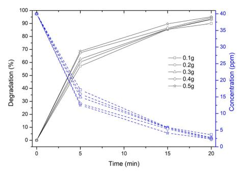
Degradation and concentration profiles of MB dye using Cu nanosheet powder of different weights under solar irradiation.
