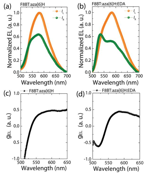
Fig. 3 Measured CP-EL spectra (a), (b) and corresponding calculated  $g_{\text{EL}}$  values (c) (d) of F8BT:aza[6]H and F8BT:aza[6]H:EDA CP-PLEDs.
