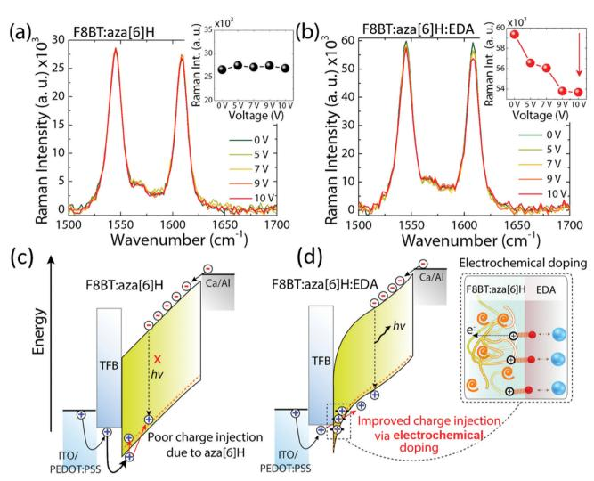
Fig. 5 (a) and (b) In situ electric-field-dependent Raman spectra of the F8BT:aza[6]H and F8BT:aza[6]H:EDA devices, respectively. The inset figures indicate the changes in the selective Raman peaks at 1608 cm<sup>-1</sup> under an electric field ranging from 0 V to 10 V. (c) and (d) The proposed mechanism of poor charge injection in F8BT:aza[6]H and improved charge injection and charge balance in an EDA-doped device via the electrochemical doping by EDA molecules (inset), respectively.
