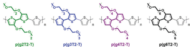
Fig. 7 Chemical structures of p(g2T2-T) , p(g3T2-T) , p(g4T2-T) , and p(g6T2-T) . Reproduced from ref. 46 with permission from the American Chemical Society.
