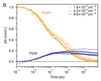
Fig. 4 (A) Schematic diagram summarising the photophysics of rubrene nanoparticles. (B) The kinetic scheme in (A) provides a good description of the singlet and triplet dynamics (residuals are shown in ESI,‡ Fig. S12). We have neglected the >100 ns triplet fusion and included singlet–singlet annihilation ( $k = 3 \times 10^{-8} \text{ cm}^3 \text{ s}^{-1}$ ) in the simulation.
