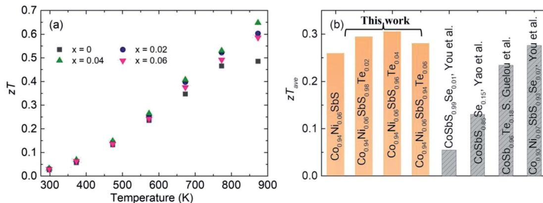
Fig. 6  $zT$  value of the  $\text{Co}_{0.94}\text{Ni}_{0.06}\text{SbS}_{1-x}\text{Te}_x$  samples ( $x = 0, 0.02, 0.04$ , and  $0.06$ ). (a) Temperature-dependent  $zT$  values and (b) comparison of the  $\text{Co}_{0.94}\text{Ni}_{0.06}\text{SbS}_{1-x}\text{Te}_x$  samples with other reported  $\text{CoSbS}$  samples prepared by Hou et al., Yao et al., and Guelou et al.
