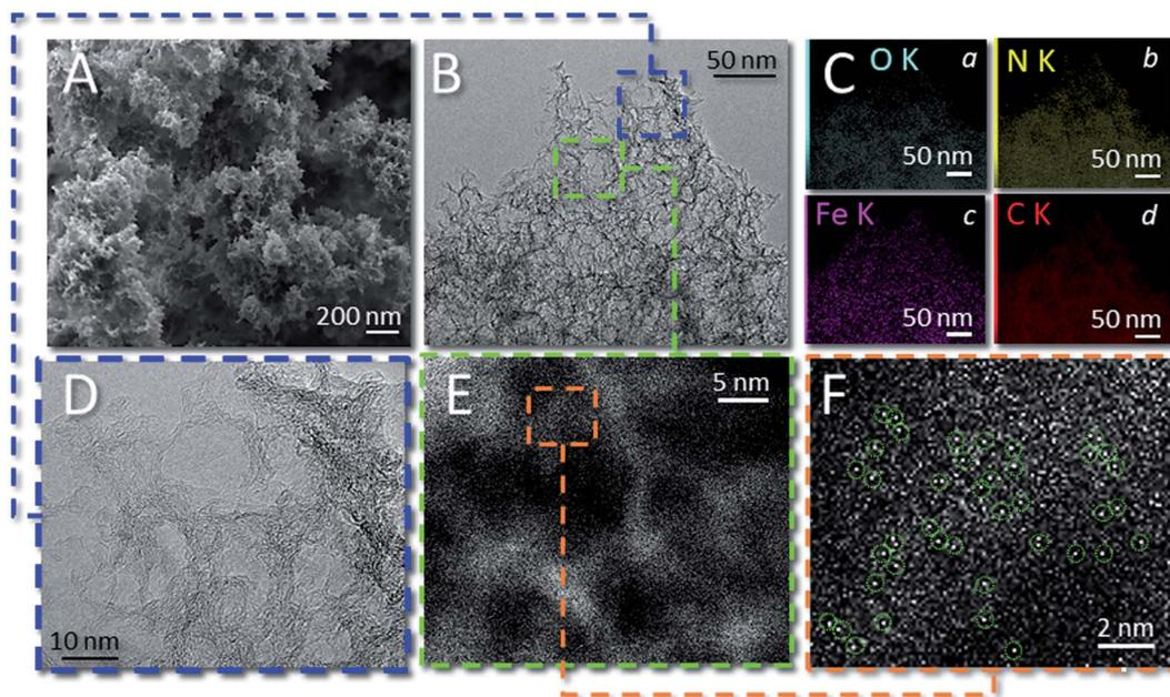
Fig. 2 (A) SEM images of **1**. (B and D) TEM images of **1** at different magnifications. (E and F) HAADF-STEM images of **1** at different magnifications. C(a–d) EDX elemental mapping for sample **1**. Color codes: C (red), N (yellow), O (light blue) and Fe (pink). (F) Highlights the bright spots assigned to heavier Fe atoms within green circles.
