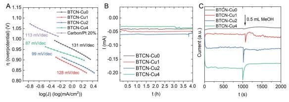
Fig. 6 (A) Calculated Tafel slopes of BTCN-Cu0, BTCN-Cu1, BTCN-Cu2, BTCN-Cu4 and Pt/C, (B) chronoamperometry curves at 0.15 V vs. Ag/AgCl (sat. KCl) over 4 hours and (C) chronoamperometry curves at 0.15 V vs. Ag/AgCl (sat. KCl) after the injection of 0.5 mL MeOH.
