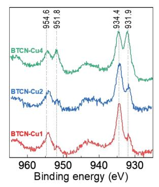
Fig. 4 Cu 2p XPS spectra of BTCN-Cu1, BTCN-Cu2, and BTCN-Cu4.
