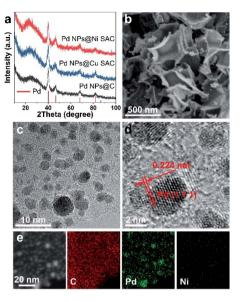
Fig. 2 Structural characterization. (a) XRD patterns of Pd NPs@Ni SAC, Pd NPs@Cu SAC, and Pd NPs@C. (b) SEM images, (c and d) TEM images, and (e) STEM images and corresponding elemental maps of Pd NPs@Ni SAC.
