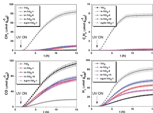
Fig. 7 Cumulative production of the main products of photocatalytic CO<sub>2</sub> reduction with the different synthesized catalysts.
