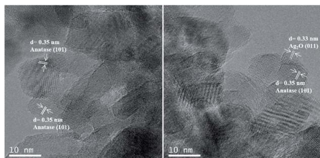
Fig. 2 TEM images of In-TiO<sub>2-1</sub> (left) and Ag/In-TiO<sub>2-1</sub> (right).
