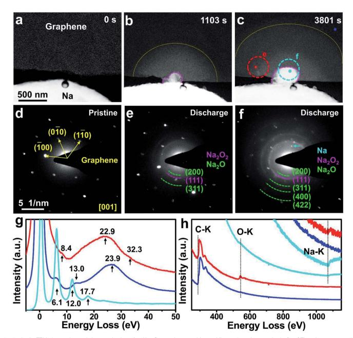
Fig. 3 In situ TEM observation and characterization of an  $Na-O_2$  nanobattery with a multilayered graphene cathode. (a-c) Time-lapse structural evolution of the graphene cathode in an  $Na-O_2$  nanobattery during the discharge process. (d-f) EDPs and (g, h) EELS of the pristine graphene and discharge products on the graphene cathode. The blue and cyan/red dots correspond to the unreacted and reacted regions, respectively.
