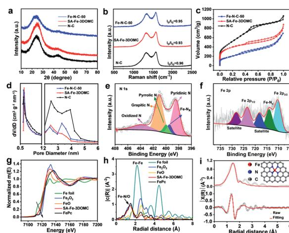
Fig. 2 (a) XRD spectra, (b) Raman spectra, (c)  $\text{N}_2$  adsorption/desorption isotherms and (d) pore size distributions of N-C, SA-Fe-3DOMC and Fe-N-C-50. (e) The N 1s high resolution spectrum of SA-Fe-3DOMC. (f) Fe 2p high-resolution spectra. (g) Fe K-edge XANES spectra and (h) Fourier transforms of the Fe K-edge EXAFS oscillations of Fe foil, FeO,  $\text{Fe}_2\text{O}_3$ , SA-Fe-3DOMC, and FePc. (i) FT-EXAFS curve fitting of SA-Fe-3DOMC in  $R$  space.
