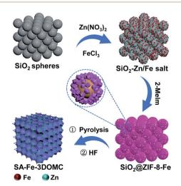
Scheme 1 Schematic illustration of the synthesis of SA-Fe-3DOMC.
