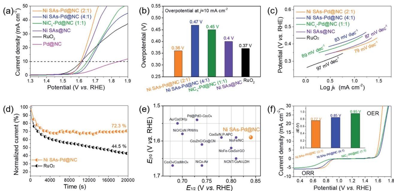
Fig. 5 (a) OER polarization curves recorded in O<sub>2</sub>-saturated 0.1 M KOH. (b) Bar plots of overpotentials obtained at 10 mA cm<sup>-2</sup>. (c) Corresponding Tafel plots. (d) Chronoamperometric curve recorded at 1.6 V. (e) Plot of comparison of catalysts from references. (f) Overall polarization curves.
