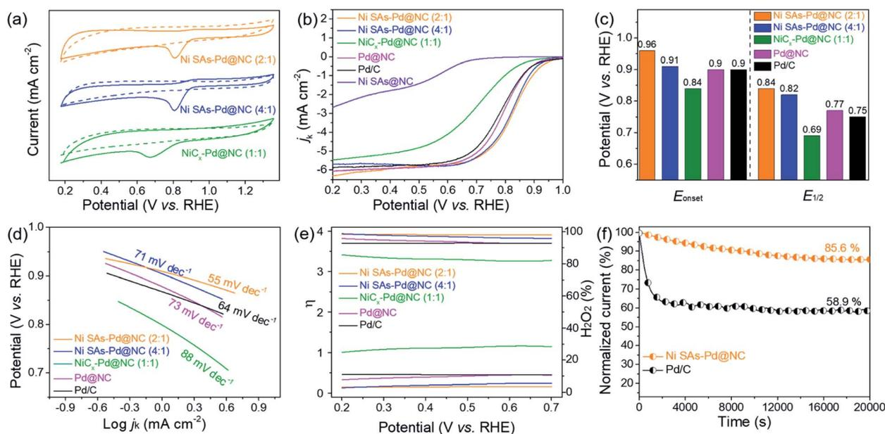
Fig. 4 (a) CV curves recorded in N<sub>2</sub> or O<sub>2</sub> saturated 0.1 M KOH solution. (b) ORR polarization curves recorded in O<sub>2</sub>-saturated 0.1 M KOH. (c) Histogram of  $E_{\text{onset}}$  and  $E_{1/2}$ . (d) Corresponding Tafel plots. (e) Curves of the average electron transfer number and percentage of peroxide. (f) Chronoamperometric curve recorded at 0.7 V.
