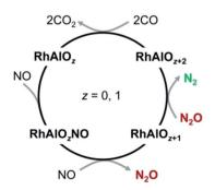
Scheme 1 Proposed catalytic cycle for the conversion of NO and CO into  $N_2$  and  $CO_2$  mediated by the neutral RhAlO $_{0-3}$  species. This catalysis can also be driven by the RhAl<sub>2</sub>O<sub>1-4</sub> clusters.
