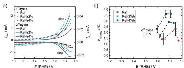
Fig. 10 (a) RRDE measurements to determine the faradaic efficiency for the OER in the overall oxidative current at  $i_{Disc}$ ,  $i_{Ring}$  was kept at 0.4 V and 0.2 V during the first and second cycle; respectively, and relates to the ORR. In (b) the faradaic efficiencies for 1 mA cm<sup>-2</sup>, 3 mA cm<sup>-2</sup> and 5 mA cm<sup>-2</sup> are provided for the 2nd scan. All measurements in N<sub>2</sub> saturated 0.1 M H<sub>2</sub>SO<sub>4</sub> at a loading of 0.13 mg cm<sup>-2</sup>.
