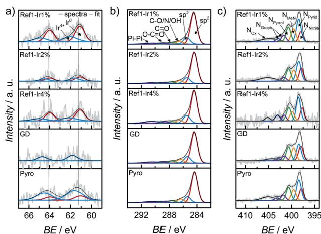
**Fig. 4** X-ray photoelectron spectroscopy (a) Ir 4f, (b) C 1s and (c) N 1s finescan regions for all catalysts modified with iridium. The dashed lines in (a) represent the position for Ir<sup>0</sup>.
