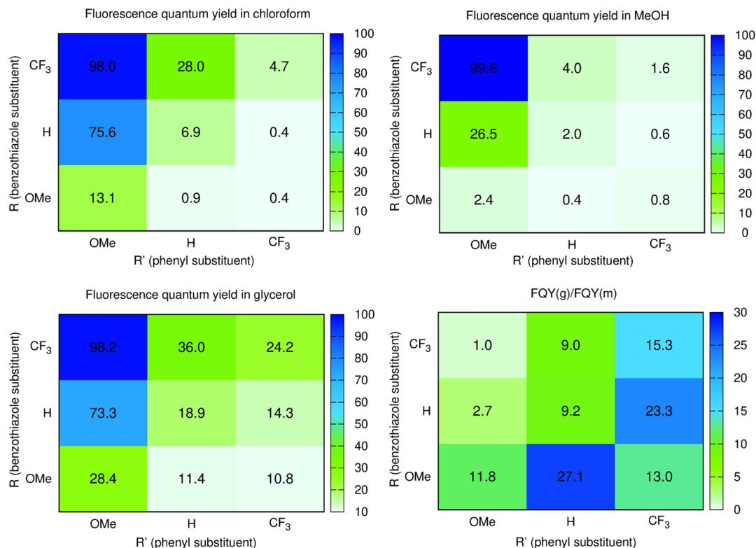
Fig. 3 Heatmaps of the fluorescence quantum yields (%) measured in  $\text{CHCl}_3$  (top left), methanol (top right), glycerol (bottom left). The bottom right figure provides the ratio between the glycerol and methanol  $\phi_f$ .
